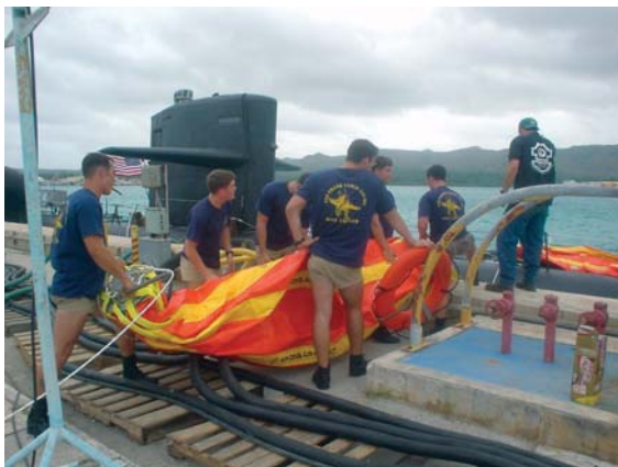
USS FRANK CABLE divers hard at work installing lift bags.
