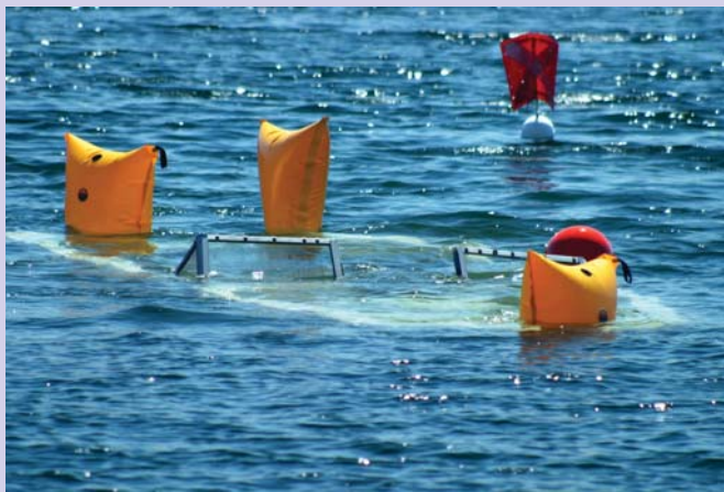
Dive Teams raise the suspect’s boat utilizing lift bags. The boat had been surveyed and videotaped by the ROVs prior to the student divers processing it on the lake bottom. Once all underwater crime scene processing was completed by Divers, the boat was recovered for further examination.
