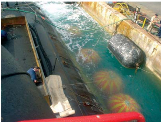
Starboard side lift bags in place.
