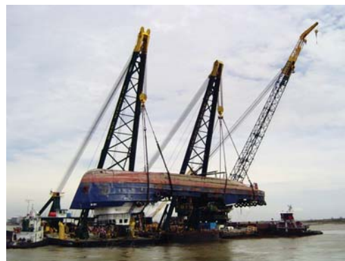
Two A-frame cranes lift the Lee III.
