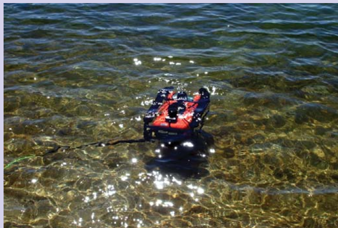
The LASD ROV is deployed from the beach in search of items of evidence lying on the lake-bed.
