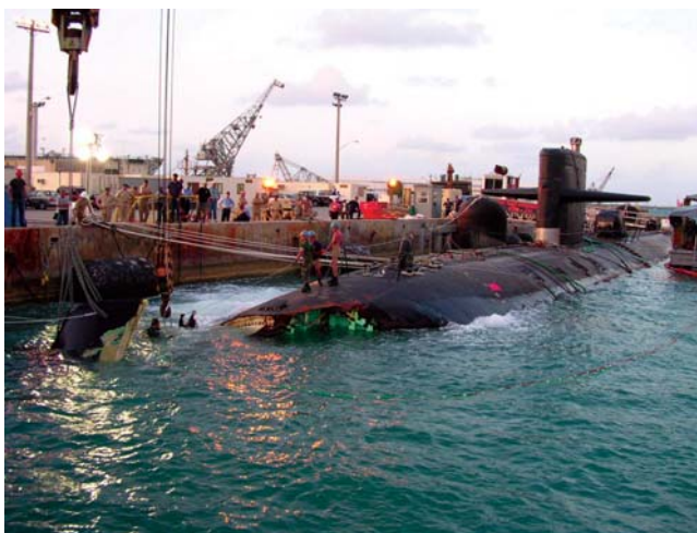
Divers removing the sonar dome.
