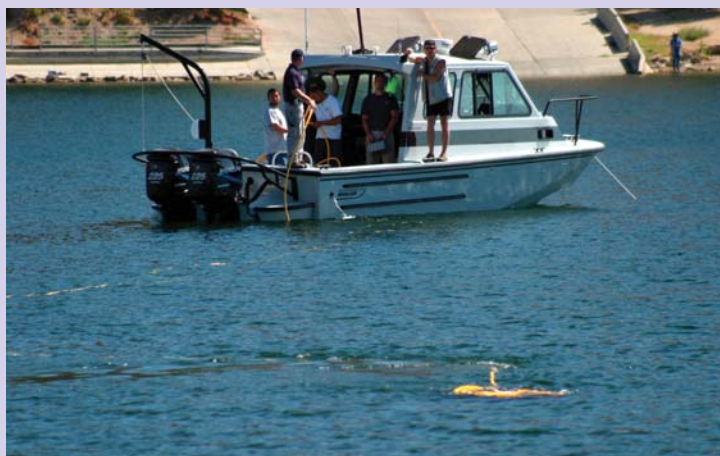
FBI Dive Team members operate the Deep Ocean Engineering Phantom 2+2. The ROV utilized its Kongsberg 650m sector scanning sonar and video camera to locate the sunken boat described by witnesses.
