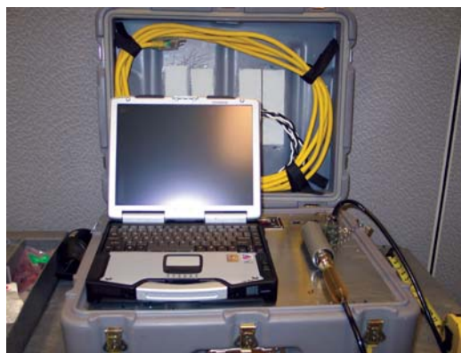
TDM with "ruggedized" components: Panasonic Toughbook computer, new pressure transducer, underwater electrical connector, and power cord in lid of container for connection to ship/shore power. If no power exists, there are two 12V batteries (lead acid) in bottom of container.
