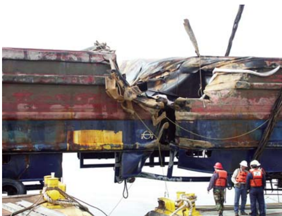
The Force of the collision is evident to onlookers surveying the hull damage as MV LEE III is lifted.
